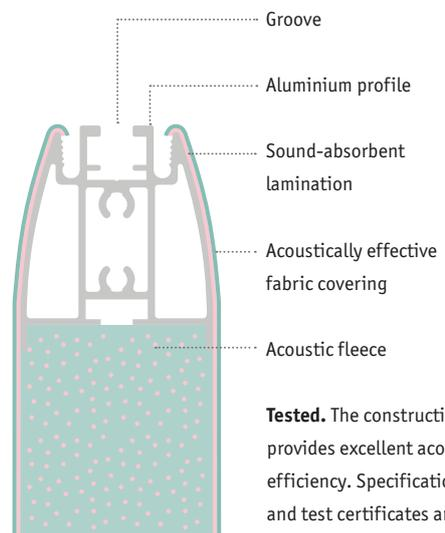
**Tested.** The construction provides excellent acoustic efficiency. Specifications and test certificates are available upon request.
